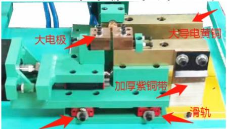
2. The integral pushing part shares 3 sets of double slider guide rails, which makes the movement easy and simple.
