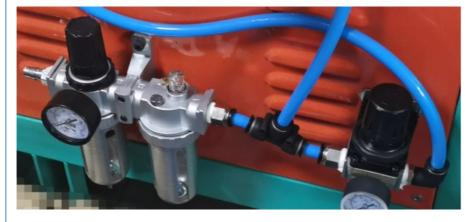
6. Taiwan SNS pneumatic components, air pipes and connectors. Independent two-piece, pressure reducing valve, convenient adjustment, oil injection, water filtration, adjustment, more independent.
