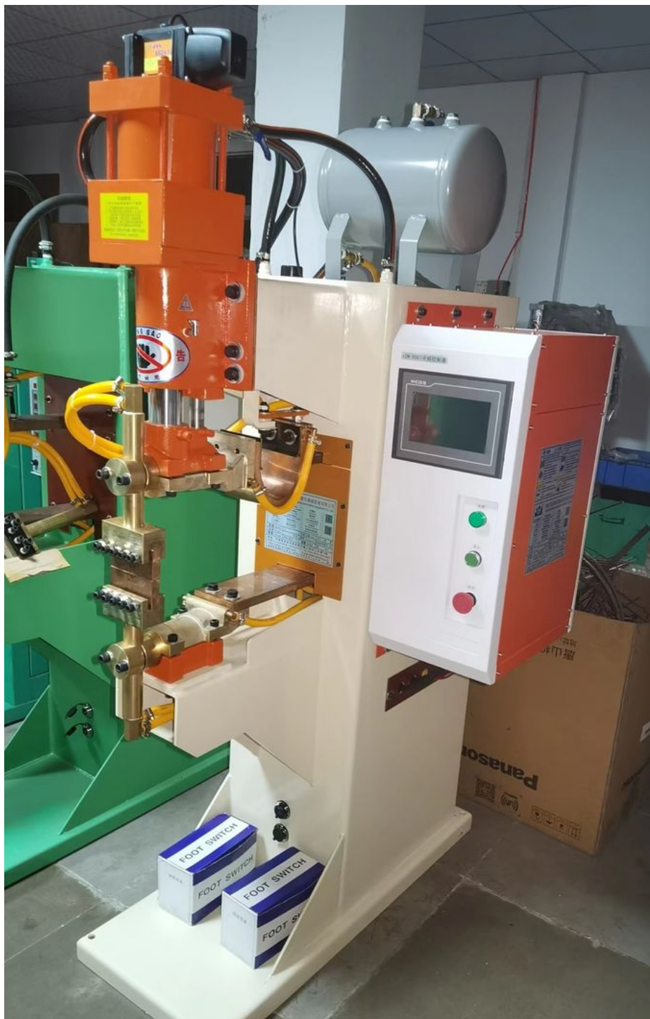
Medium frequency row welding machine, mainly used for stainless mesh, multi spot welding. The welding is firm and the surface is beautiful.
