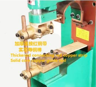
3. Taiwan Yadeke AIRTAC solenoid valve, precision electric control box and module thyristor are better than similar configurations, with more stable and soft welding current, small spark and more beautiful welding surface.
