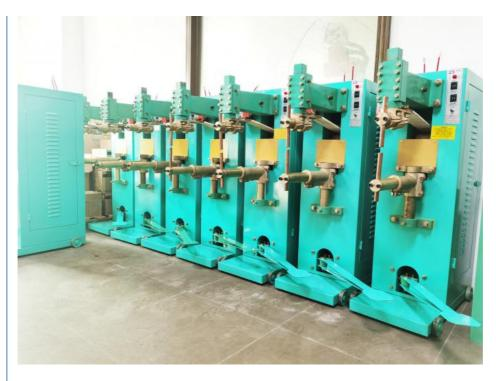
This spot welding machine is the simplest and fully mechanical. It is carefully designed and equipped with perfect accessories. Within the welding range, the welding effect can be achieved very well. Compared with the pneumatic spot welding machine, it requires foot strength when working. The operator will work harder and the efficiency will be slower.
