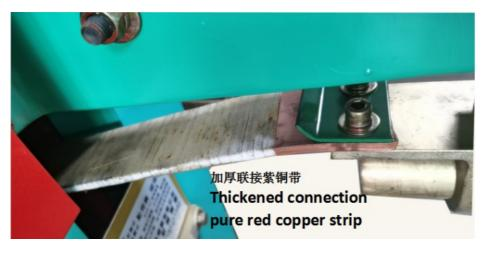
5. Solid conductive copper rod with good conductivity. The pull rod is connected with copper base, 380V current is connected, stable and durable. Transformer red copper coil and high-grade silicon steel sheet. The transformer has strong current, sufficient capacity and stronger welding ability. It is not easy to oxidize for a long time and the welding is more stable.
