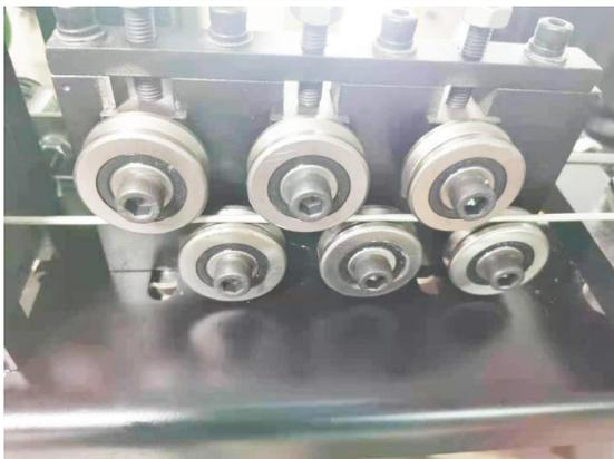
2. 4 groups, 8 wire feeding forming wheels, with large force, stability and wear resistance. There are only 3 groups and 6 similar machines from other manufacturers. Moreover, the processing is accurate, and the surface of the trunking is specially smooth.
